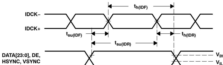
**Figure 2. Control and Single-Edge-Data Setup/Hold Time to IDCK±**
