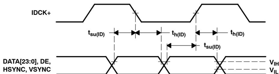
**Figure 3. Dual Edge Data Setup/Hold Times to IDCK+**
