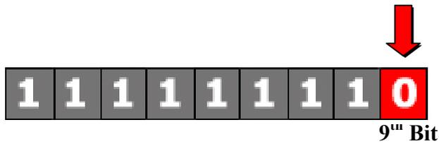
**Figure 12: No TM Encoding Required**
