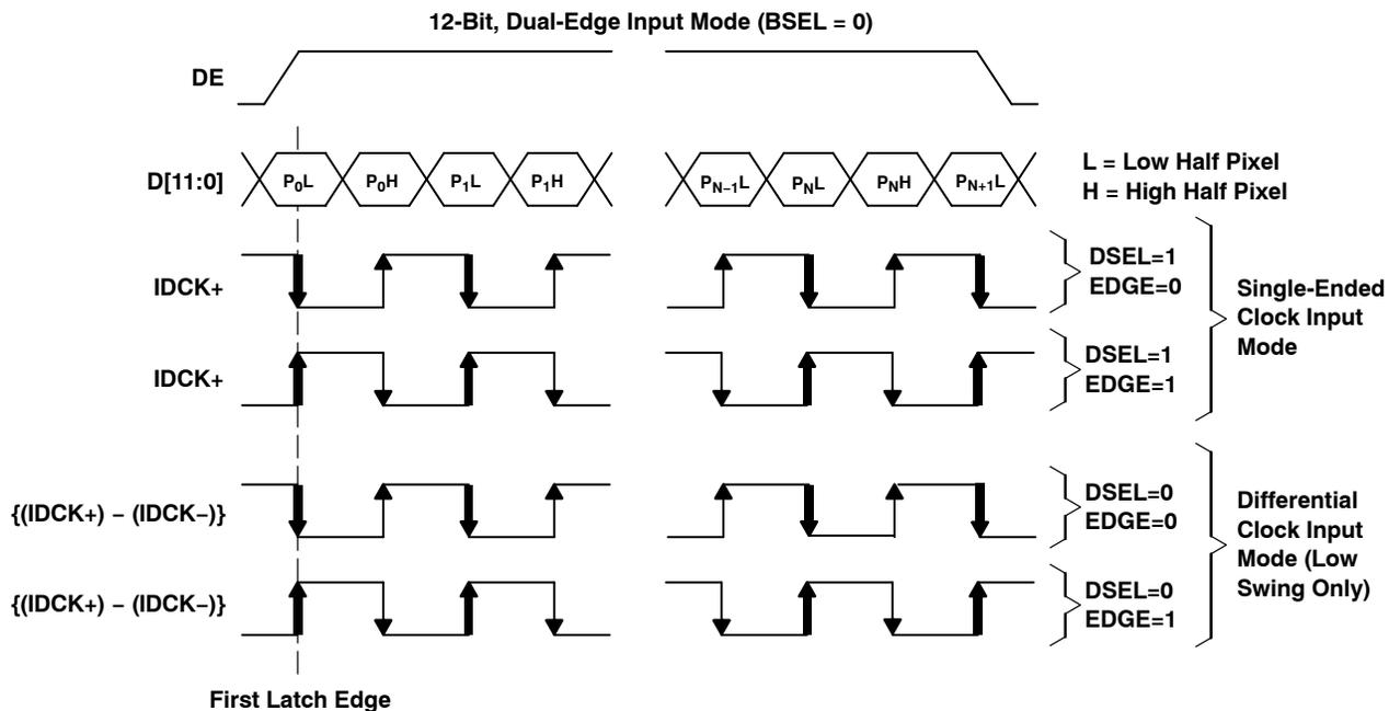
**Figure 6. Universal Graphics Controller Interface Options for 12-Bit Mode (Graphical Representation)**
