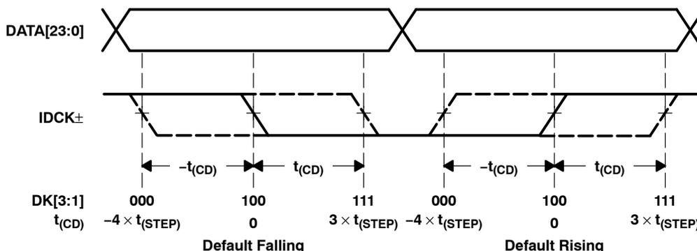
**Figure 8. A Graphical Representation of the De-Skew Function**
