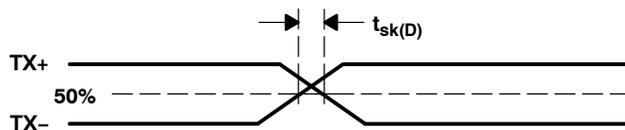
**Figure 4. Analog Output Intra-Pair ± Differential Skew**
