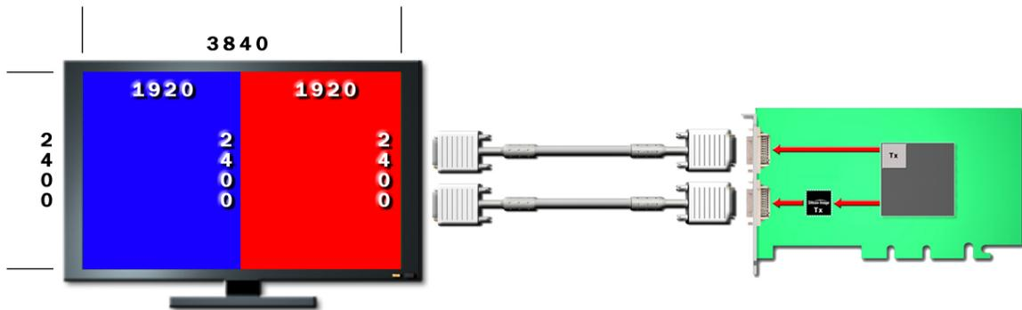
**Figure 29: Two Single-Link DVI Ports Driving a 9 Megapixel Display**
