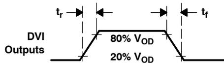
**Figure 1. Rise and Fall Time for DVI Outputs**
