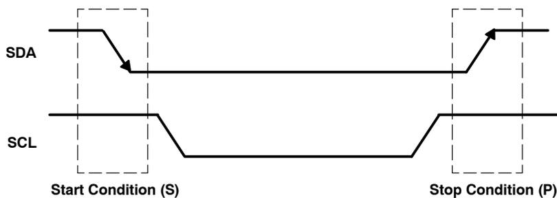
**Figure 10. I<sup>2</sup>C Start and Stop Conditions**
