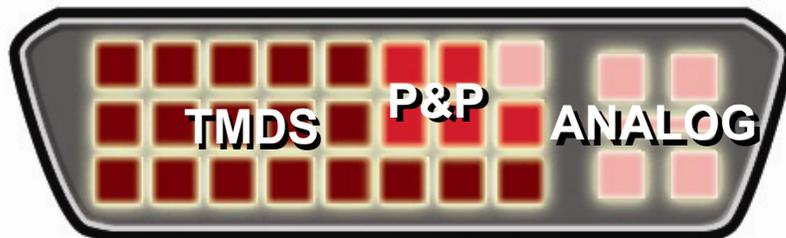
Figure 20: TMDS, Plug & Play and Analog Signals
