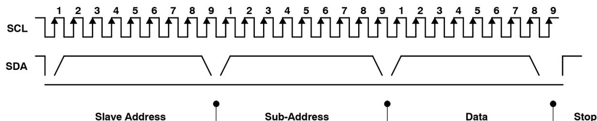
**Figure 11. I<sup>2</sup>C Access Cycles**
