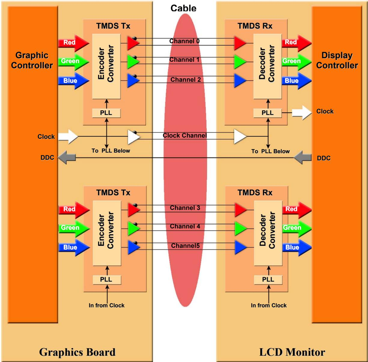
Figure 6: Dual-Link DVI. Although not shown, both transmitter PLLs are linked together, as are the receiver PLLs.
