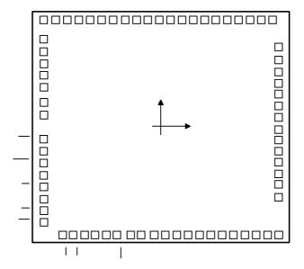
${Chip~size:~155\times148~(mil)}^2 \\ *~The~IC~substrate~should~be~connected~to~VDD~in~the~PCB~layout~artwork. }$
