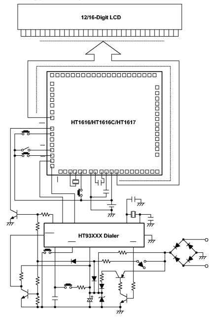
$<sup>\</sup>ensuremath{^{*}}$  The IC substrate should be connected to VDD in the PCB layout artwork.
