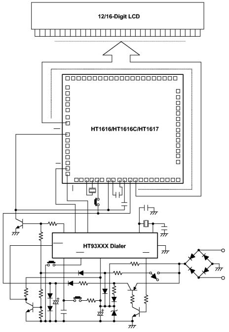
$\ensuremath{^{*}}$  The IC substrate should be connected to VDD in the PCB layout artwork.
