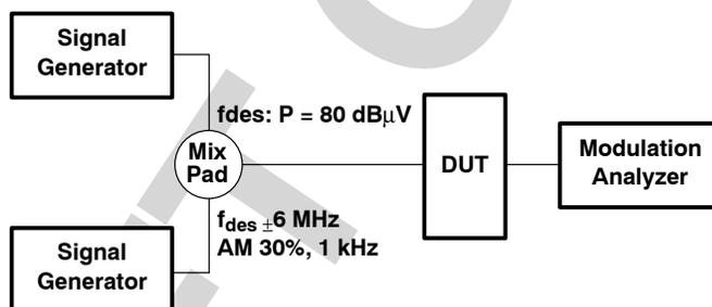
Figure 17. 1% Cross Modulation Distortion Measurement Circuit
