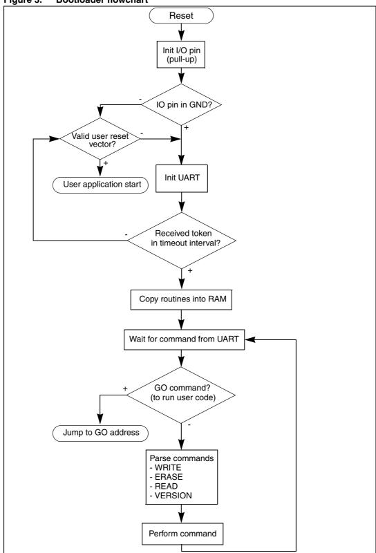
Figure 3. Bootloader flowchart
