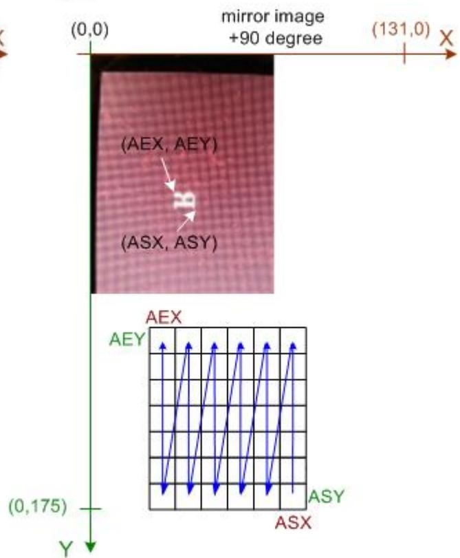
The given programming sequences are using the definition of the picture writing routine above. Note that the width (CHAR\_W) and the height (CHAR\_H) have to be swapped, if the image is displayed in a 90 degree rotation. Initial, before starting data writing and address mode changing, the register have to be defined and the addressing mode has to be set using the following code sequence:
