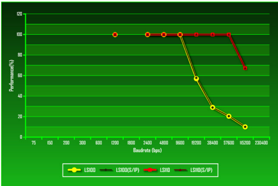
Figure 6: Throughput Test Result of Lite Series – TCP/IP vs. Serial/IP
