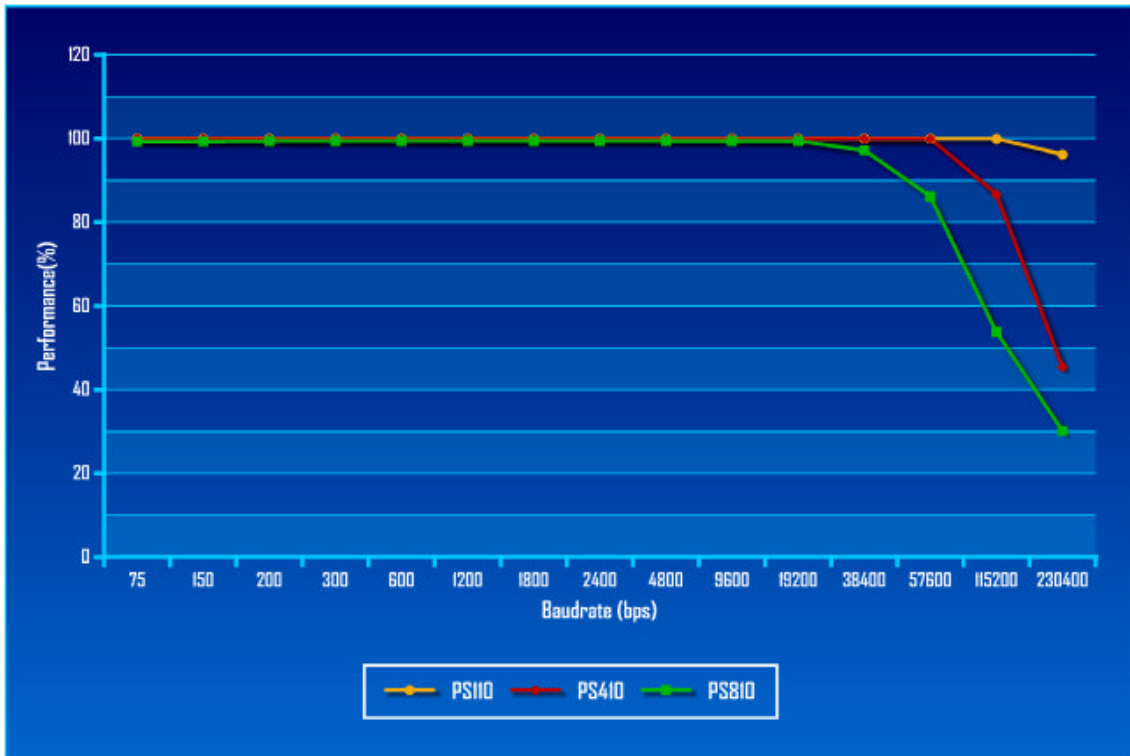
Figure 7: Throughput Test Result of Pro Series
