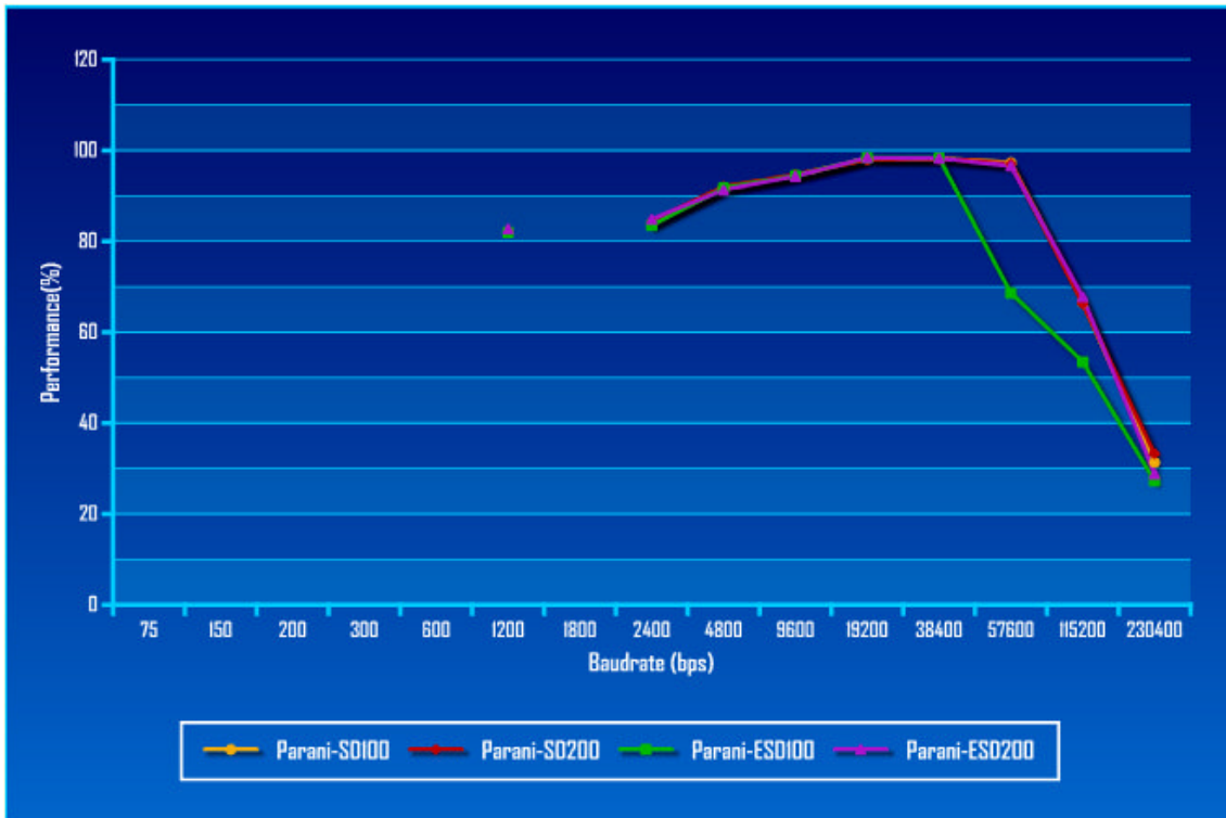
Figure 11: Throughput Test Result of Bluetooth-Serial Adapters
