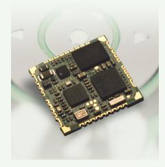
The **eMD3620F** ezRide -22 module is housed in a 22.0 x 3.0 mm SMD package that includes all the required components for a complete GPS/AGPS solution.
