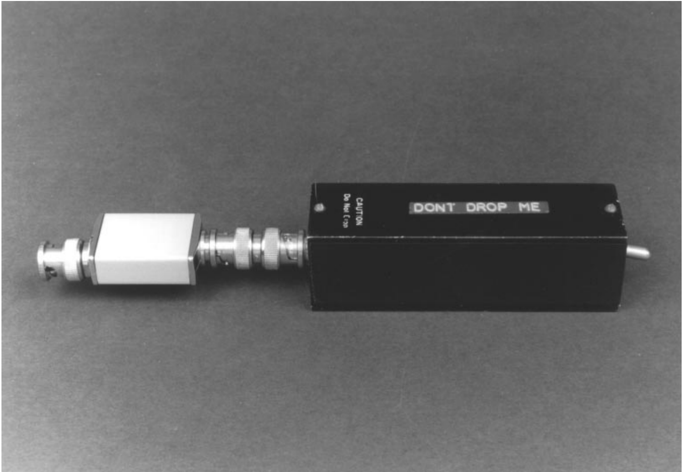
Figure D4. The Packaged Avalanche Pulser. 1.5V-90V Converter is in the Black Box. Avalanche Head is at Left
