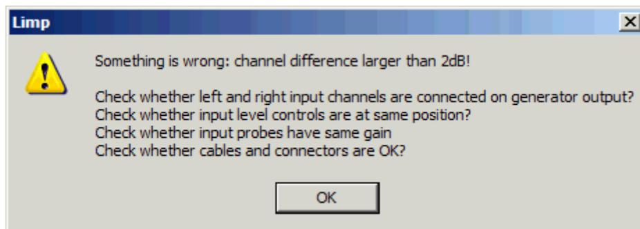
**Figure 4.21** Report when channel difference is larger than 2dB.
