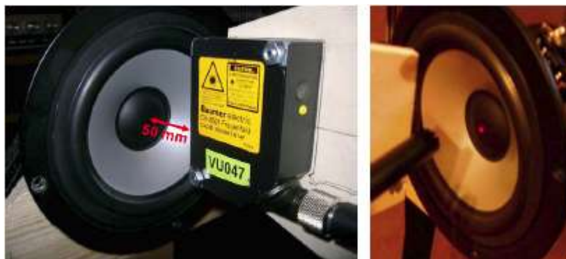
Figure 3.7. Positioning of laser displacement sensor and microphone
