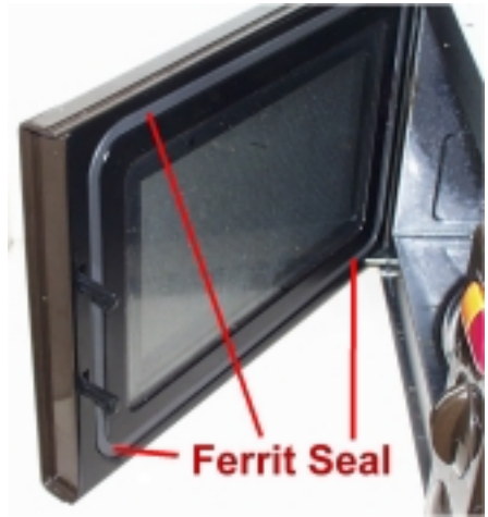
The magnetic sealing integrated in the door
