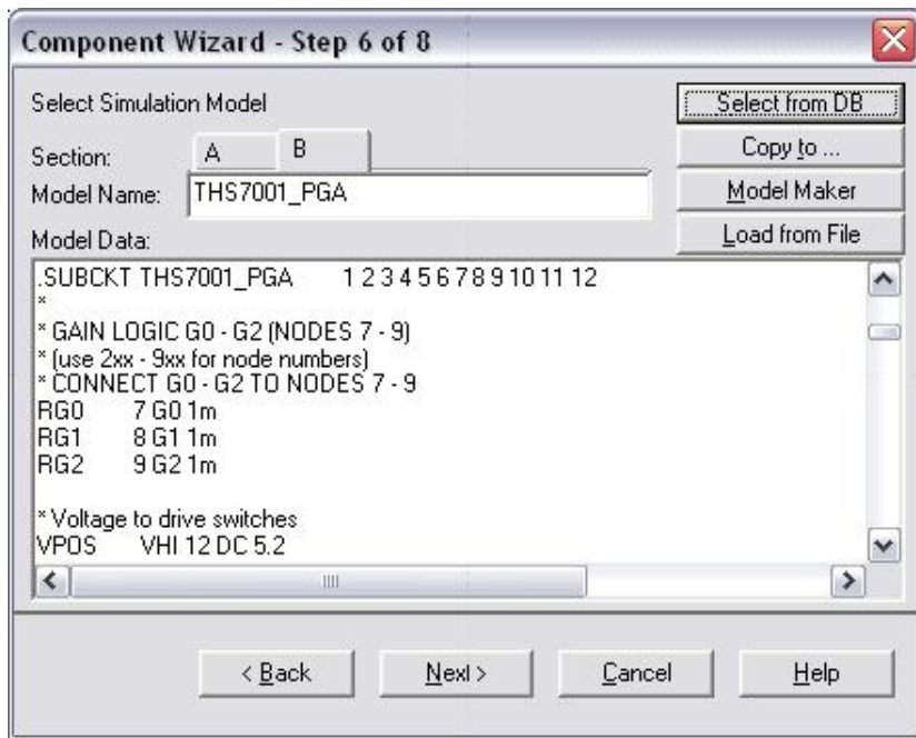
Figure 11 - SPICE Model for THS7001 PHA Stage
