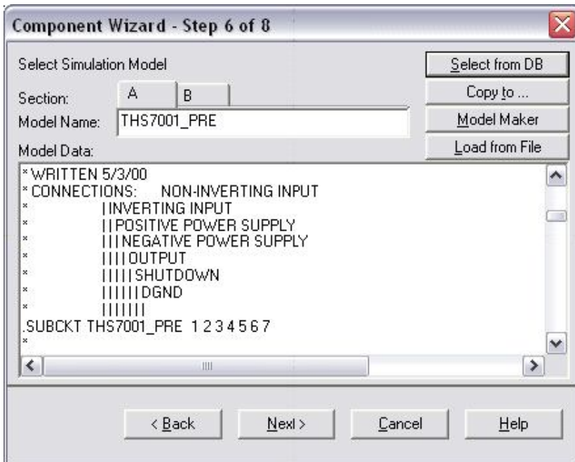
Figure 10 - SPICE Model for THS7001 Preamp Stage
