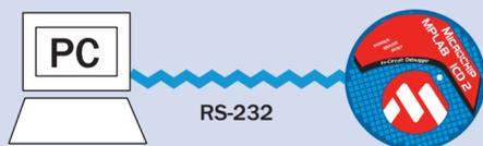
2. Select the COM port to set up for communication, i.e., *Control Panel>System>Hardware>Device Manager>Ports>COMx*, (where x = 1, 2, 3, etc.), right-click on the desired COM port, and select Properties.
