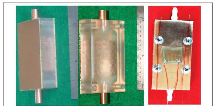
Figure 4. Double and single sided see through functional cold plates (left), top view of the single sided test unit (right).
