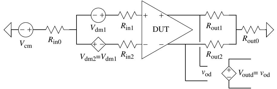
that maps between two distinct ground-referred signals and a balanced pair of signals. The two distinct signals would represent the differential- and common-mode components of the balanced signals. Thus, if  $v_d$  and  $v_c$  represent the distinct signals representing the differential- and common-mode components, and  $v_p$  and  $v_n$  make up the balanced pair of signals, then
