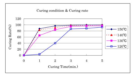
Thermal analysis : DSC (Differential Scanning Calorimetry)
