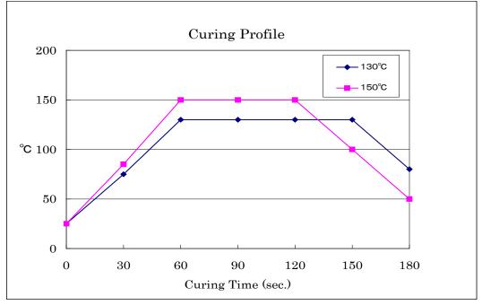
In a case that large devices are laid near or on the back of the dispensed adhesive, the great calorific capacity of these devices would absorb heat to consequently give rise to phenomenon that additional longer curing time are needed.
