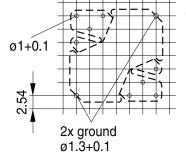
Hole arrangement View in mounting direction
