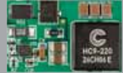
LT3755: Boost Demo Circuit. Actual Size, Complete Solution
