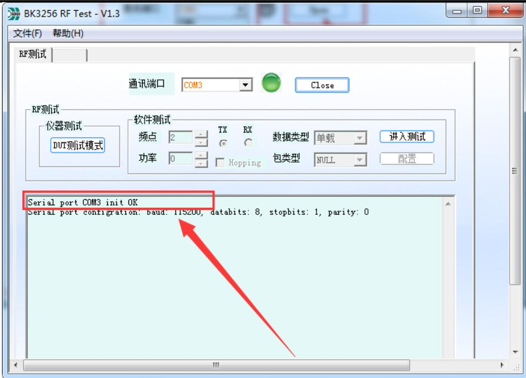
5. Maintain the state of connection between the certification machine and the test equipment, turn on the power to turn on the working state of the certification machine, the connection is normal as shown below.
