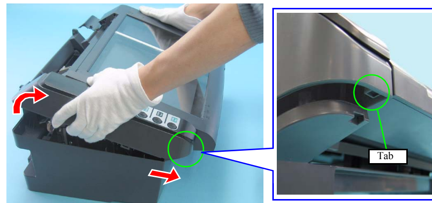
Figure 4-15. Removing Scanner Unit /Middle Case /Panel Unit (5)
