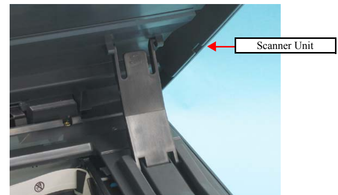
Figure 4-8. Installing Support Arm
