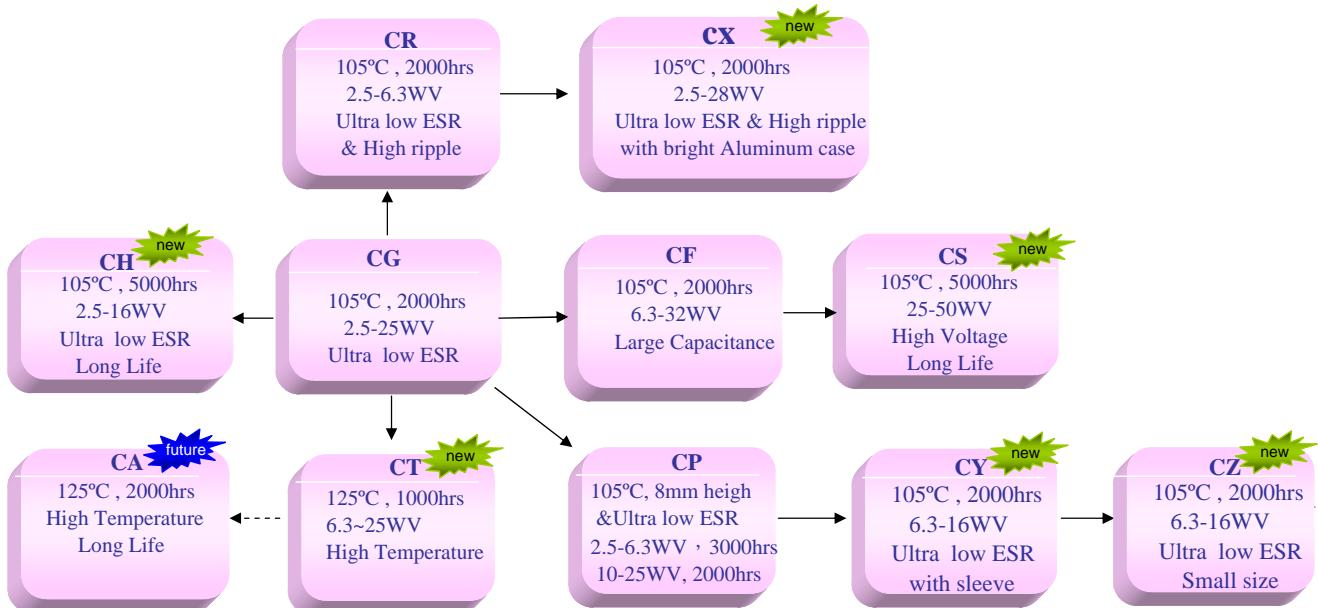
**Conductive Polymer Aluminum Solid Capacitors :SMD**
