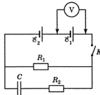
$$U = U_0 \frac{\frac{\mathcal{E}_2 + r_2}{R_1 + r_1} + \frac{\mathcal{E}_1 + r_1}{R_2 + r_2}}{\frac{\mathcal{E}_2 + r_2}{R_1 + r_1} + \frac{\mathcal{E}_1 + r_1}{R_2 + r_2} + 1} = 9,8 \text{ В}; U = U_0 \frac{\frac{\mathcal{E}_2 + r_2}{R_1 + r_1}}{\frac{\mathcal{E}_2 + r_2}{R_1 + r_1} + \frac{\mathcal{E}_1 + r_1}{R_2 + r_2} + 1} = 3,6 \text{ В}$$
