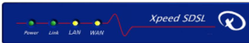
The X320R has four LEDs on the front to indicate system status.
