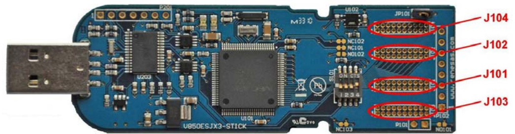
Figure 6 External connectors J101, J102, J103 and J104
