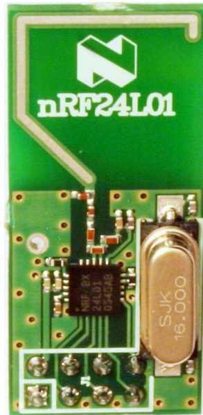
Figure 1: The nRF24L01 Reference Module with PCB antenna and a HC49 crystal
