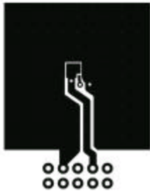
a) 56^\circ\text{C}/\text{W} when mounted on a 1\text{ in}^2 pad of 2 oz copper
