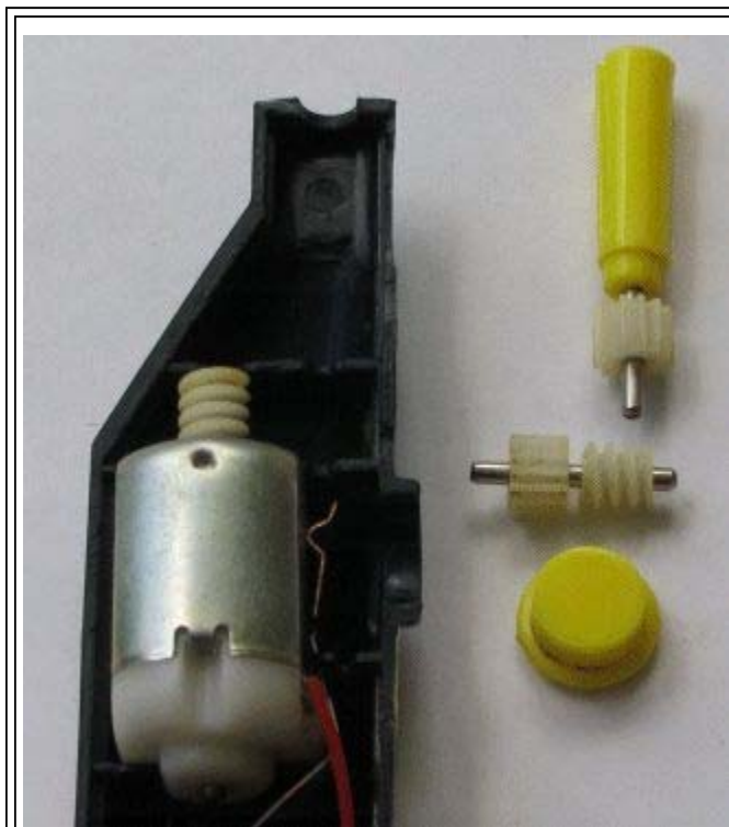
A two-worm reduction gearbox producing a reduction of 12:1 and 12:1 = 144:1 The gears are in the correct positions to produce the reduction.
