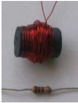
Inductor: 60 turns on 10mm ferrite rod, 15mm long.
