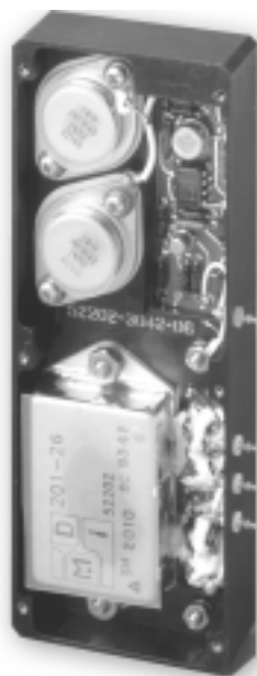
Figure 22: Power Converter using a combination of a hybrid module and outboard discrete components for fast lead time and low development cost. Unit shown is a 14 to 28 VDC converter with 90% efficiency at 40 Watts.
