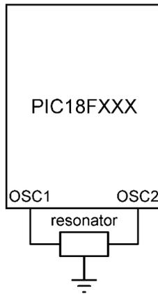
Figure 2.15: Using a resonator as the clock input
