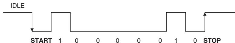
**Figure 6.50: Sending character “A” in serial format**
