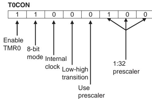
Thus, T0CON register should be loaded with hexadecimal  $0 \times C4$ . The next register to be configured is the interrupt control register INTCON, where we will disable priority based interrupts and enable the global interrupts and TMR0 interrupts:
