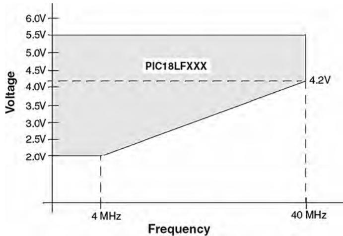
Figure 2.10: Operation of PIC18LF452 at different voltages
