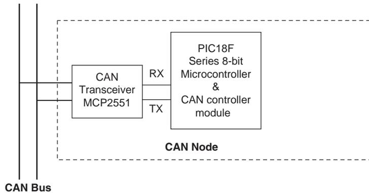
Figure 9.12: CAN node with integrated CAN module
