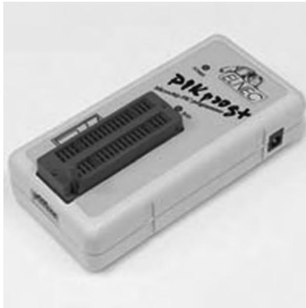
**Figure 5.16: PIC Prog Plus programmer**
