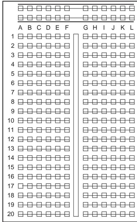
**Figure 5.25: Internal wiring of the breadboard in Figure 5.24**
