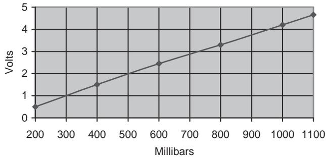
**Figure 8.35: Variation of sensor output voltage with pressure**
