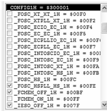
Figure 8.24: Selecting clock bits for USB operation
