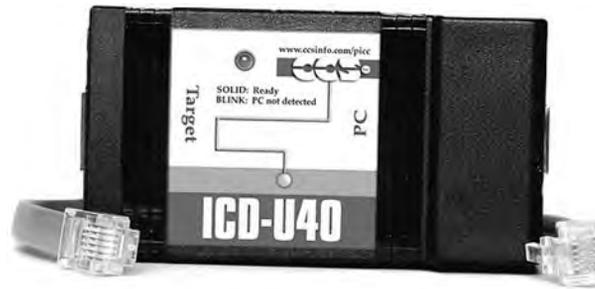
Figure 5.18: ICD-U40 in-circuit debugger
