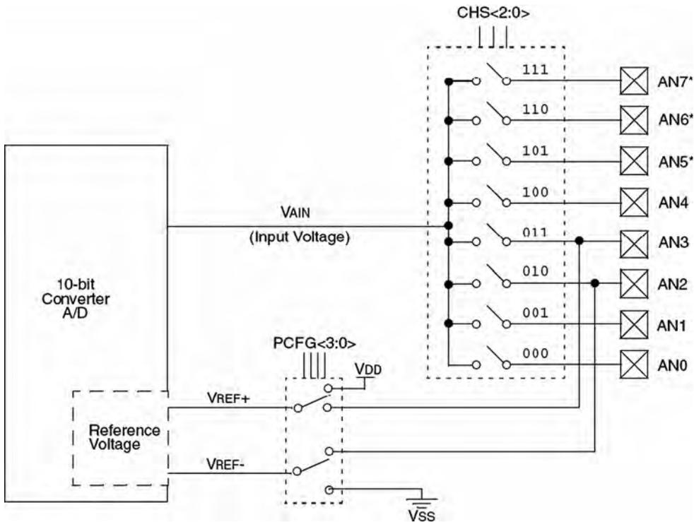
**Figure 2.41: Block diagram of the PIC18F452 A/D converter**
