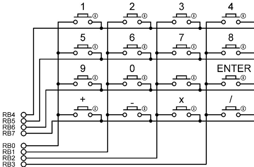
Figure 6.44: 4 × 4 keypad structure
