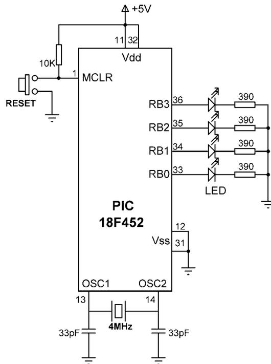
**Figure 10.7: Circuit diagram of the project**
