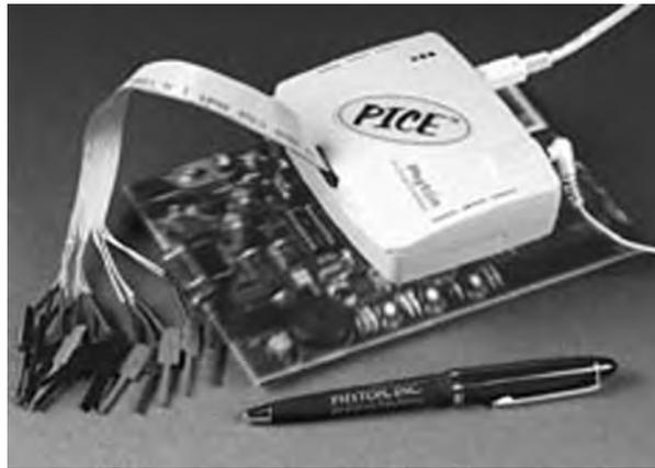
**Figure 5.23: PICE-MC in-circuit emulator**
