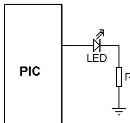
**Figure 4.15: Connecting the LED in current sourcing mode**
