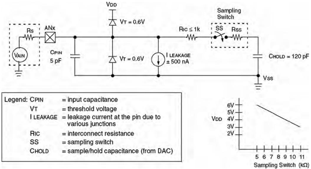
**Figure 2.45: Analog input model of the A/D converter**
