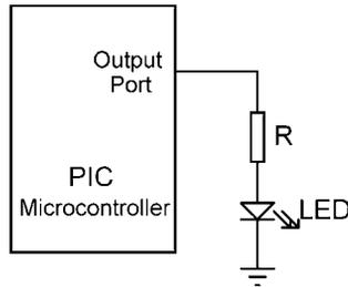
**Figure 6.2: LED connected in current sourcing mode**
