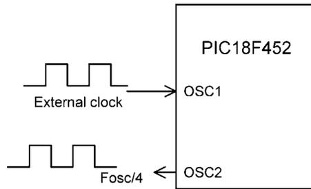
**Figure 2.17: External clock in EC mode**
