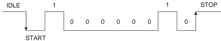
**Figure 4.21: Sending character “A” in serial communication**
