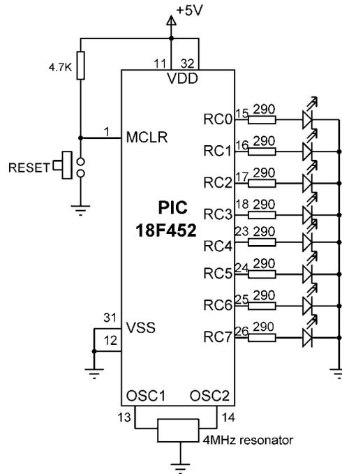
Figure 6.3: Circuit diagram of the project
