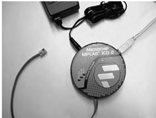
**Figure 5.17: ICD2 in-circuit debugger**
