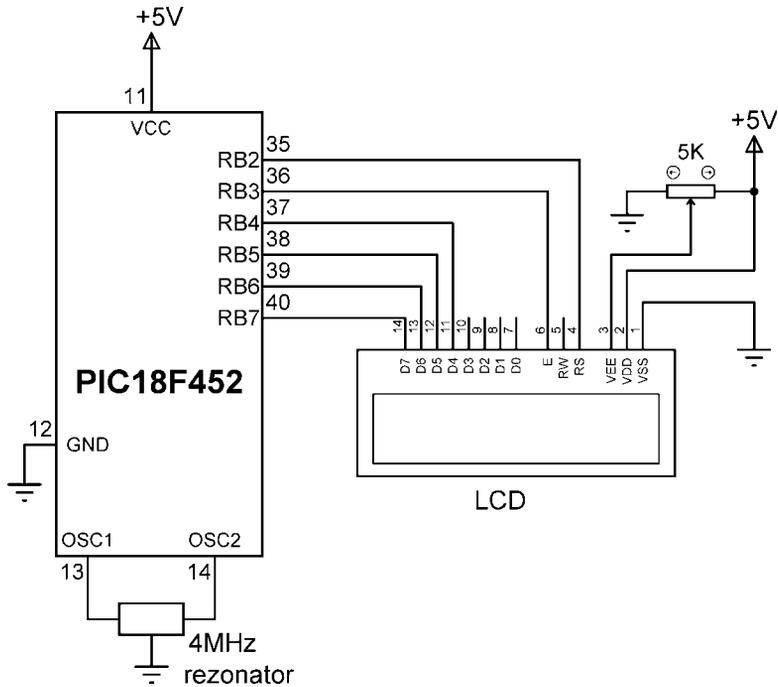
**Figure 4.19: Connecting an LCD to a PIC microcontroller**
