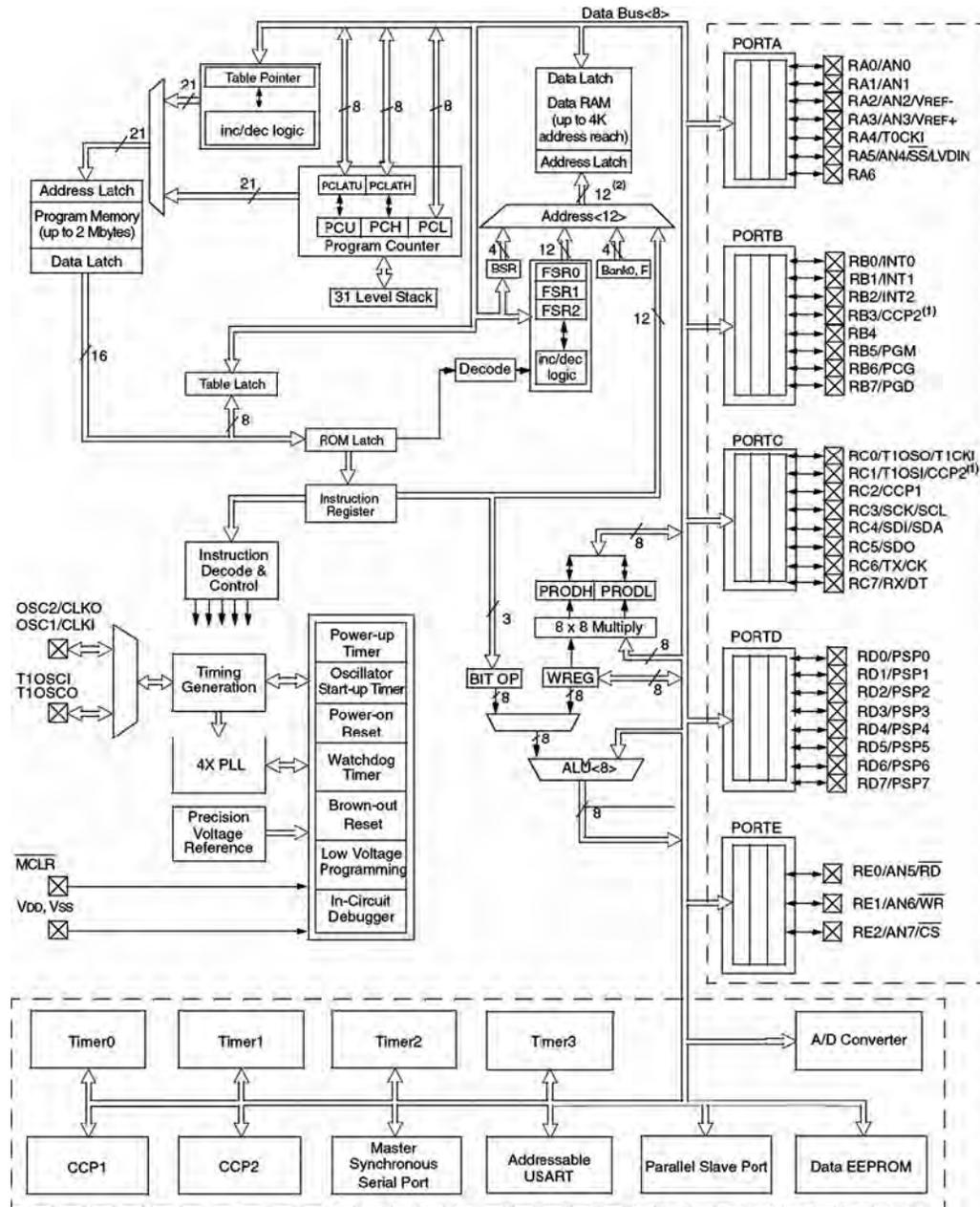
Figure 2.2: Block diagram of the PIC18F452 microcontroller
