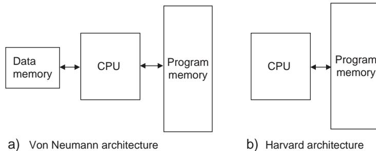
**Figure 1.4: Von Neumann and Harvard architectures**
