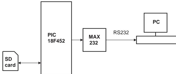
**Figure 7.7: Block diagram of the project**
