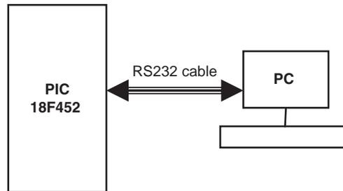
**Figure 6.53: Block diagram of the project**
