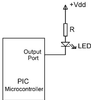
**Figure 6.1: LED connected in current sinking mode**
