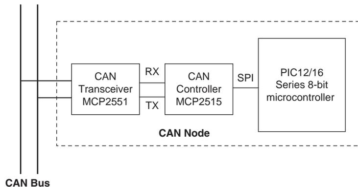
Figure 9.11: CAN node with any PIC microcontroller
