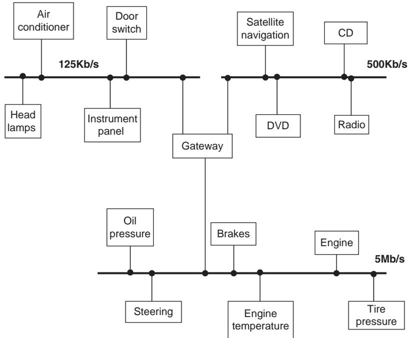
**Figure 9.1: Typical CAN bus application in a vehicle**
