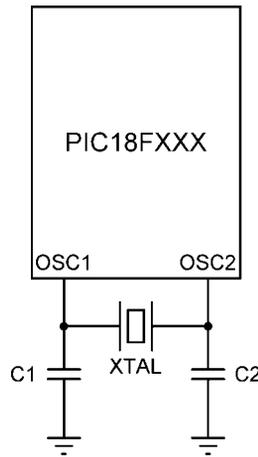
**Figure 2.14: Using a crystal as the clock input**
