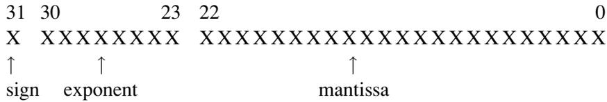
The most significant bit indicates the sign of the number, where 0 indicates the number is positive, and 1 indicates it is negative.
