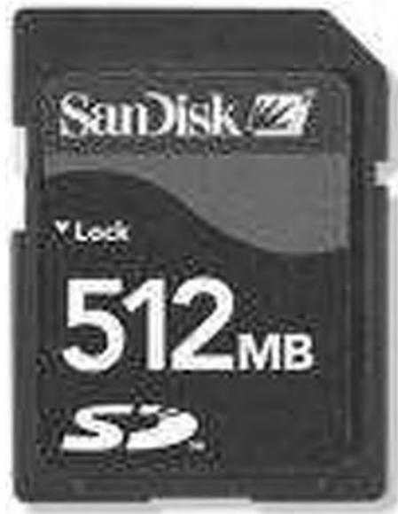
Figure 7.1: A typical SD card
