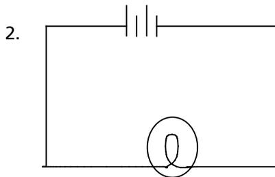
Here is the electrical diagram of a circuit that includes a battery and a light bulb. They are connected to each other by wire. Build this circuit and get the light bulb to light up.
