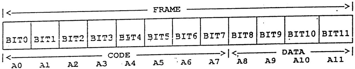
The input data is encoded by the AX5326 and sent out serially four times through the DOUT pin for each low pulse on the TE pin. The data encoding format is as follows:
