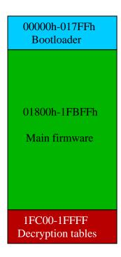
Of the three memory areas ,only the two can be updated. The entire 128Kbytes of flash memory is divided in blocks of 1kbyte each, so we have 128 blocks numbered from 0 to 127 as follows:
