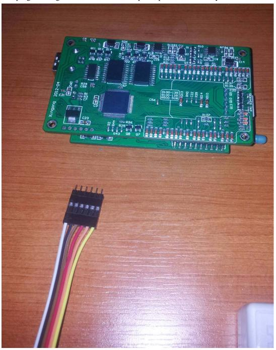
In this image the TL866 programmer is reflashed by another TL866, be sure to activate ICSP\_VCC enable in the minipro software.
