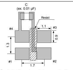
To maintain stable operation, provide by-pass capacitor with more than 0.1  $\mu F$  at a location as near as possible to the power source terminal of the crystal products (between VCC - GND).
