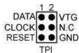
The ISP header is used for standard 8bit avr devices, the PDI header for the newer XMEGA AVRs and the TPI header for the 6-pin TINY AVRs.
