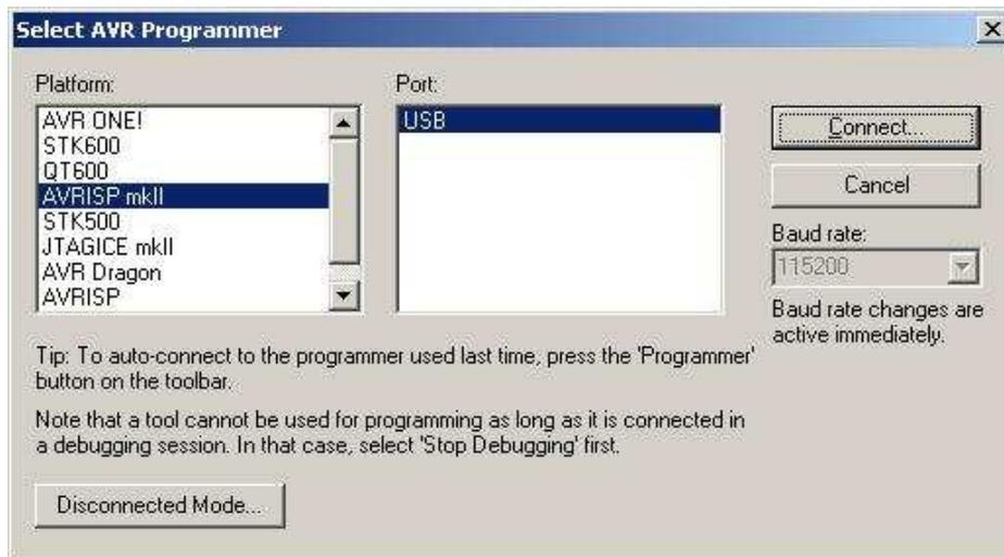
Once connected the device selection menu will pop up. Connect the programmer cable to the appropriate header to flash the target device depending on target device selected. Be sure your target device is 5v tolerant if you select the USB powered mode.
