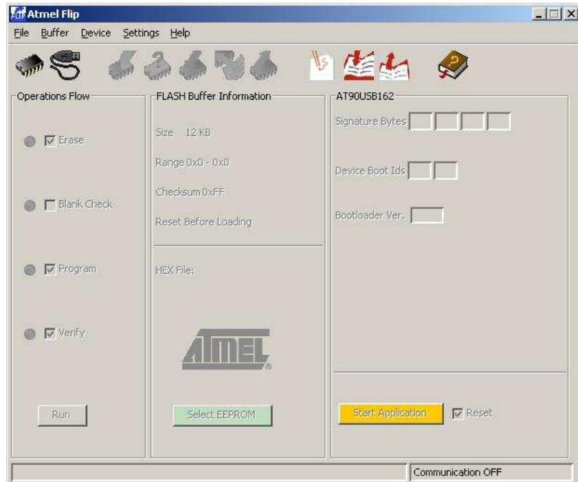
Click on the 'chip' icon or 'Device → Select' menu option and select the device from the dropdown menu (at90usb162).
