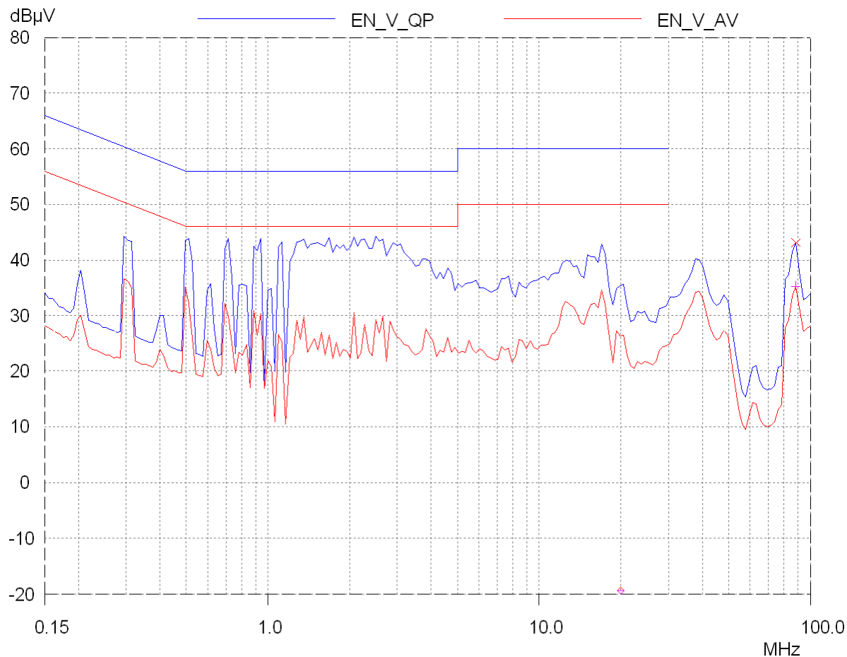
Figure 38 – Conducted EMI, 230 VAC.
