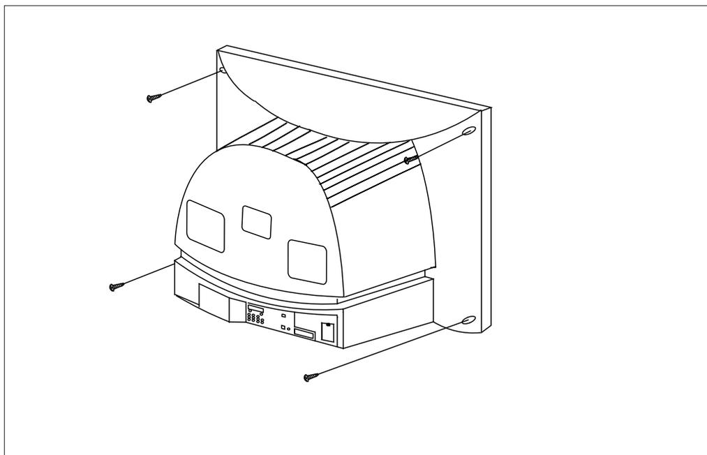
1. After removing the screws, press the tension rib and pull the cabinet backwards.
