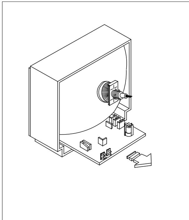
1. Separate the socket board from the CRT neck.
