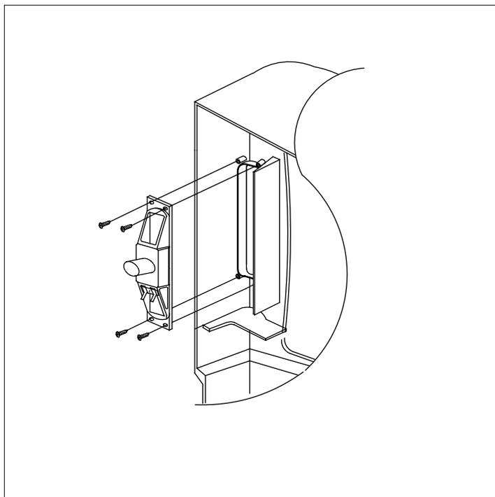
1. Remove the speaker by pressing the tension rib.
