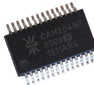
Figure 2 CAM204 28-pin SSOP
