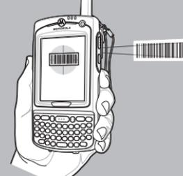
1. Launch a bar code reading application on the MC75A.
