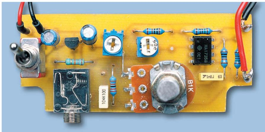
Check your completed PC board assembly carefully to ensure that all polarised components have been correctly installed. These parts include IC1, REG1 and the two electrolytic capacitors.
