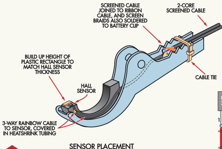
Fig.5 (above): this exploded diagram shows how the toroid core and Hall sensor are fitted to the clamp. Each core half is secured in position using builders' adhesive, as are the Hall sensor and the adjacent plastic rectangle. Note the earth connection to the metalwork of the clamp.
