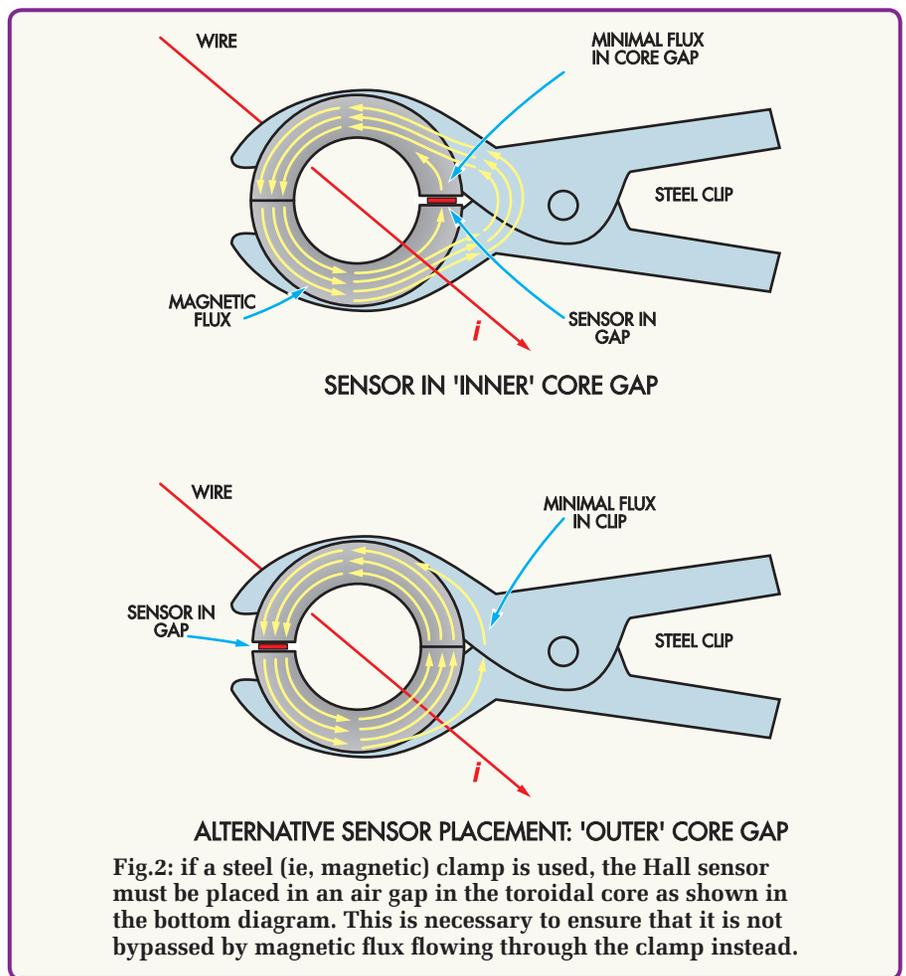
**Fig.2: if a steel (ie, magnetic) clamp is used, the Hall sensor must be placed in an air gap in the toroidal core as shown in the bottom diagram. This is necessary to ensure that it is not bypassed by magnetic flux flowing through the clamp instead.**
