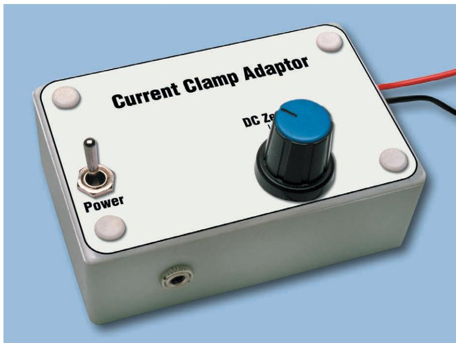
There's no power LED on the front panel to warn you when the power is on, so be sure to switch the unit off when it is not in use to save battery life. Also, be sure to null the reading on the multimeter (ie, when there is no current flow through the core) before taking a measurement.
