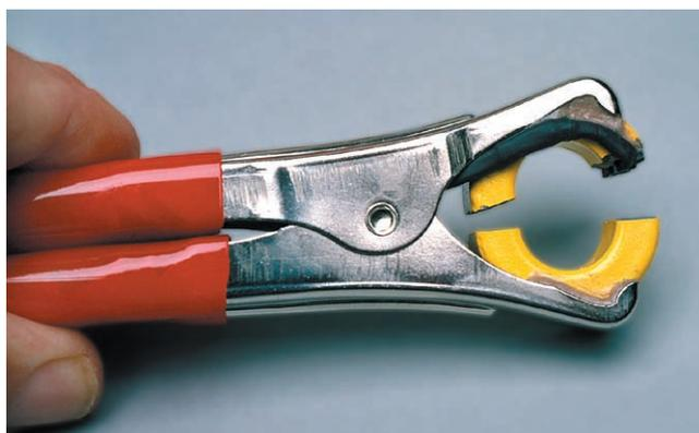
This view of the completed current clamp clearly shows the general arrangement. If the toroid core becomes magnetised during use, it can be demagnetised by momentarily reversing the current flow in the core.
