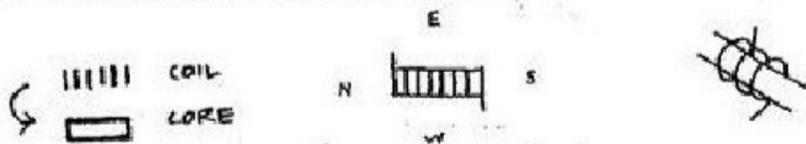
When you pushed the coil to the middle of the field magnet, the North Pole magnet current came out of the wire end that is pointing East, and the South Pole magnet current came out of the wire end that is pointing West, but when you pushed the coil away from the middle of the field magnet the currents reversed, then North Pole magnet current came out of the coil's wire end that is pointing West and South Pole magnet current came out of the coil's wire end that is pointing East.
