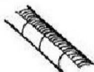
Now the wire in the coil is one continuous magnet. One side of the wire is South Pole and the other North Pole.
