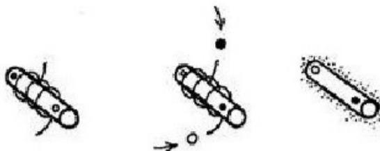
When you were pushing the coil through the U shaped magnet you got two flashes in the light bulb with one passage through the U shape magnet, and I showed you from which ends of coil's wire the currents came out while they made the flashes.
