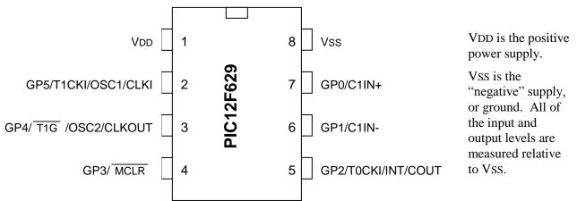
In most circuits, there is only a single ground reference, at 0 V, and VSS will be connected to ground.
