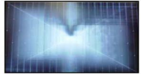
Solder defect, Short/Crack
