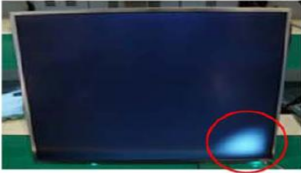
Panel Mura, Light leakage
