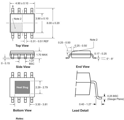
1. All dimensions in millimeters; angles in degrees
