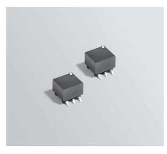
These surface mount transformers are designed for high switching speed, transformer coupled MOSFET and IGBT gate drive circuits operating from 50 kHz to as high as 2 MHz. They offer low leakage inductance, excellent interwinding capacitance and 1500 Vdc primary to secondary isolation.
