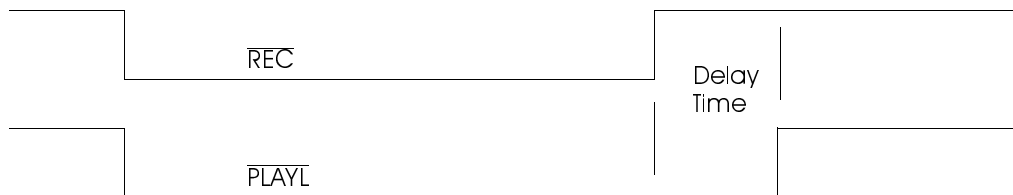
Figure 1: Delay Time from \overline{\text{REC}} to \overline{\text{PLAYL}} Rising Edges
